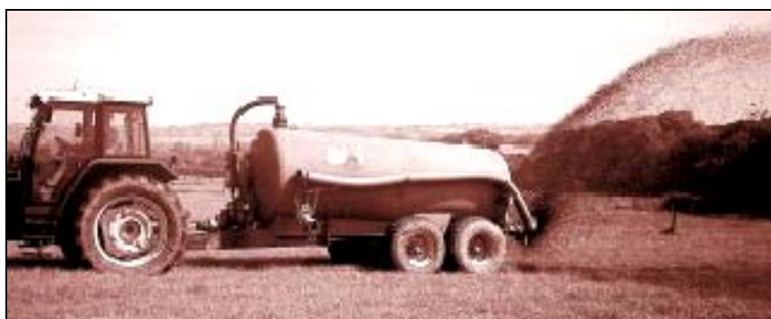
Figure 2.36: Example of a broadcast spreader with a splash plate [51, MAFF, 1999]
