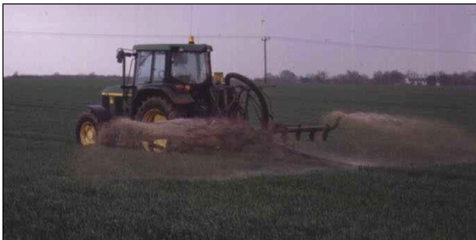
Figure 2.38: Example of a broadcast technique with low trajectory and low pressure [220, UK, 2002]
