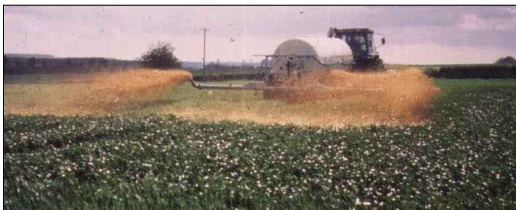
Figure 2.39: Example of a broadcast technique with low trajectory and low pressure [220, UK, 2002]
