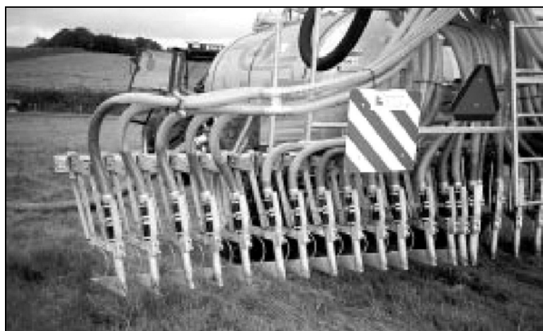
Figure 2.41: Example of a trailing shoe spreader [51, MAFF, 1999]
